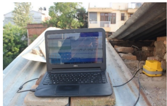
Figure 3. Data Collection at site. The highest point accessible in the mid longitudinal wall
